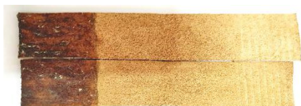
Fig. 5. Shear strength test for prepared bio-adhesives
