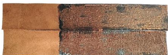
Fig. 6. Peel strength test for prepared bio-adhesives
