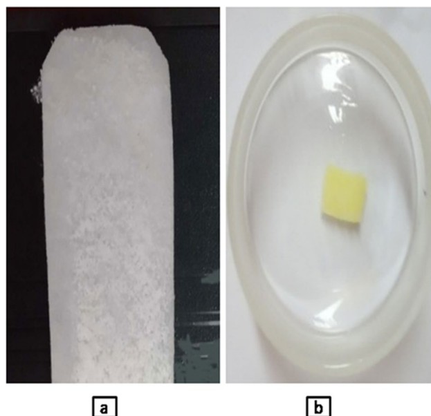
Fig. 1 Sulfonated GMA-g-PE a before adsorption, b after U(VI) adsorption
