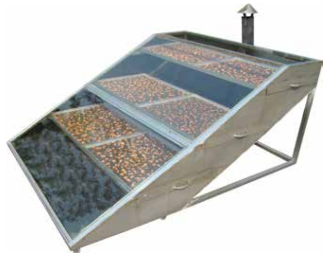
Fig. 4. Pictorial view of Solar dryer for large production
