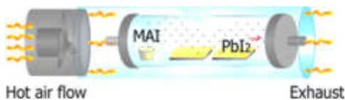
Fig. 22. Schematic diagram of the ambient atmosphere vapour-assisted deposition method.
