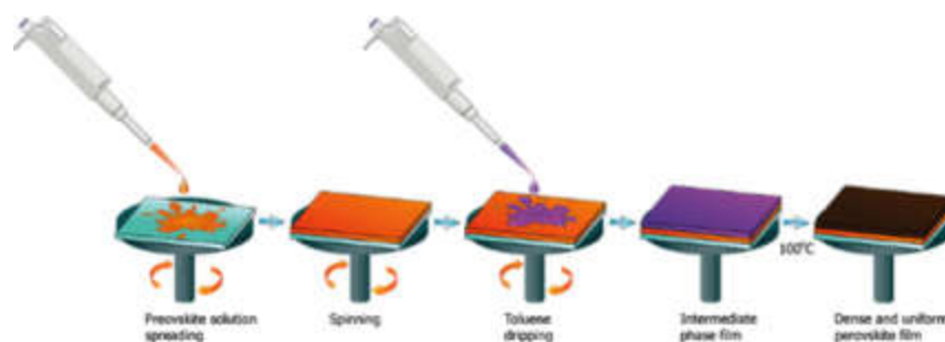
Fig. 4. Simple representation of anti-solvent treatment for the OSD technique.
